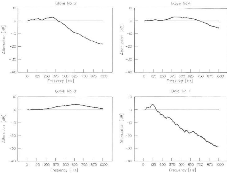
FIG. 3. Attenuation provided by gloves Nos 3, 4, 8 and 11 as a function of frequency.
