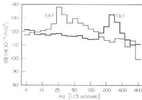
FIG. 4. One third octave band weighted spectra according to ISO 5349. (a) Chipping hammer and (b) pneumatic grinder.
