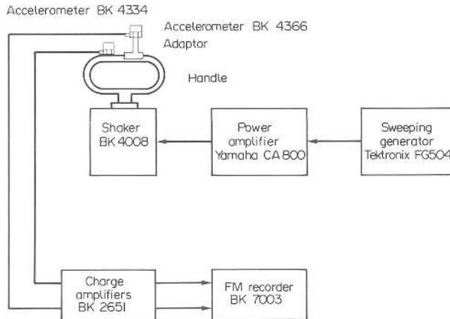
FIG. 1. Set-up used for testing gloves.
